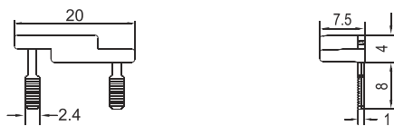
S1D-B1, 10A @ 250 VAC, 1 Way Bridge for Coil
